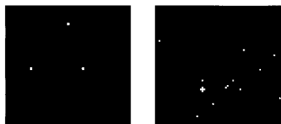
Figure 2. Subframe images ( 50 \times 50 pixels) of fluorescence from the reaction product. Left: fluorescamine concentration of 1 \times 10^{-6} M at 4'55", and right: fluorescamine concentration of 1 \times 10^{-5} M at 4'30". Other experimental conditions and cutoff threshold selections remain the same as in Figure 1.
